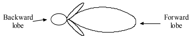
Figure 1.5 Radiation pattern of a directional antenna
