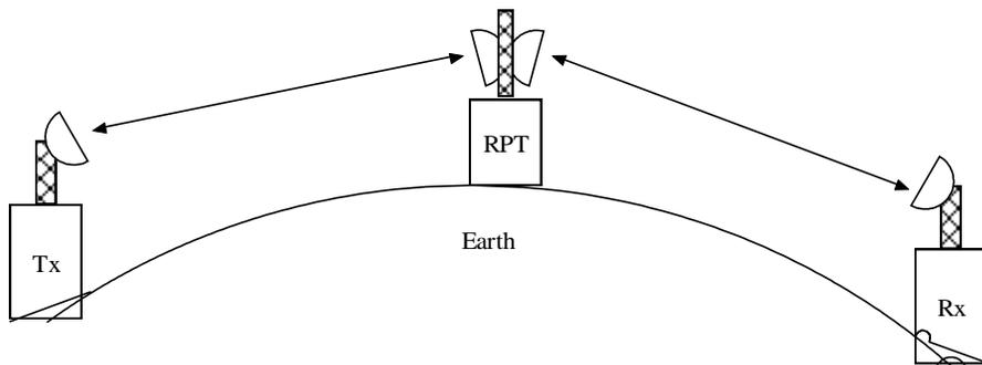
Figure 5.1 Microwave radio relay link
