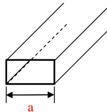
**Figure 5.6** Rectangular waveguide
