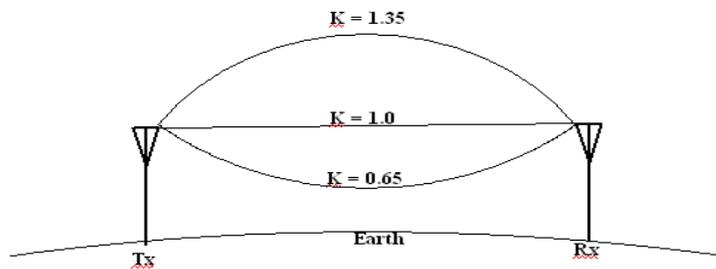
Figure 5.4 Propagated ray trajectories for different values of  $K$
