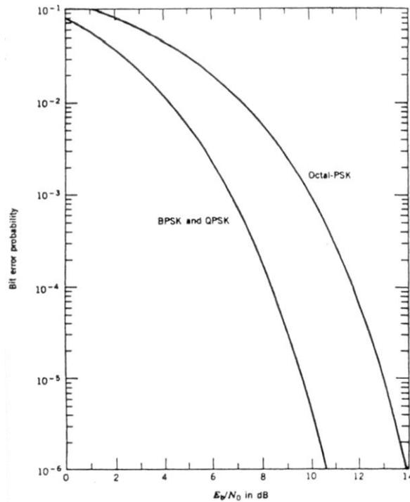
**Figure 5.5** BER versus  $E_b/N_0$  performance curve BPSK, QPSK and Octal PSK
