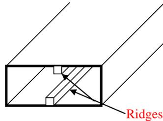
**Figure 5.5** Ridge waveguide
