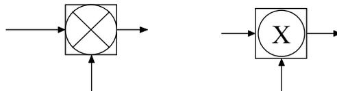
Figure 2.6 Balanced modulator symbols
